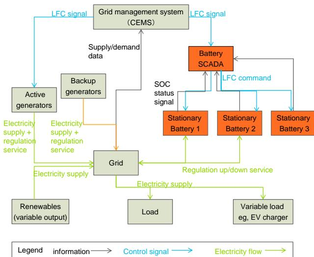
**Figure 1. Battery SCADA schematic**
