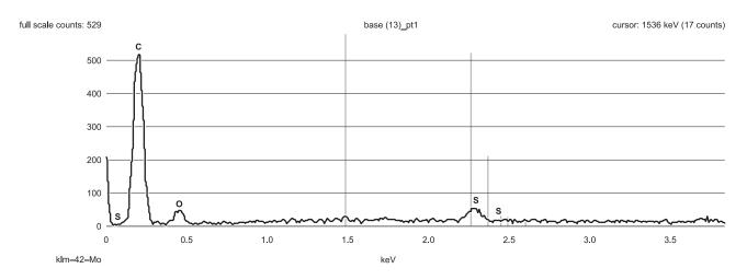
Fig 144 Energy-dispersive spectrum of a representative region of the wax scrapings (C - carbon; O - oxygen; S - sulphur)
