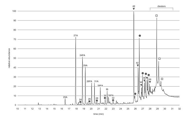
Fig 142 Partial high temperature gas chromatogram showing distribution of components of trimethylsilylated lipids identified from the wax on stylus tablet <WT108>: xA-n-alkane with carbon chain length x; xFA – free fatty acid with carbon chain length x; IS – internal standard; filled squares – n-alkanols with carbon chain length shown; filled triangles – palmitate alkyl esters with carbon chain length shown; filled circles – hydroxy wax esters; open squares – palmitate diesters
