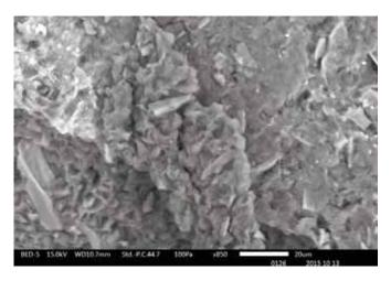
Fig 143 Back-scattered electron image of a representative region of the wax scrapings
