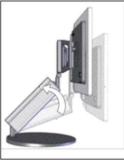
Figure 2: Adjusting the support column
