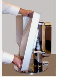
Figure 3 Tilting a Flat Panel
